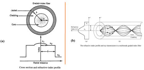
Figure 15: Graded index fiber
