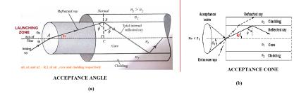
Figure 13: Propagation of light inside optical fiber
