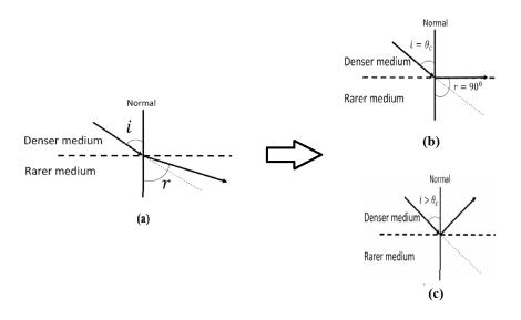
Figure 10: Total internal reflection
