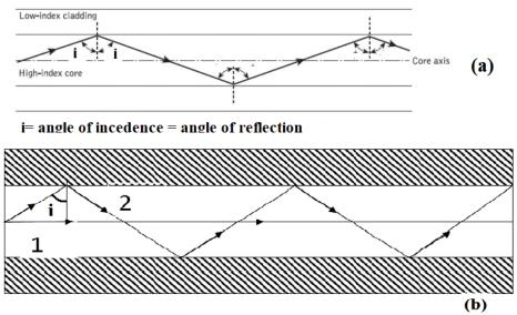
Figure 12: Light ray suffering series of total internal reflection inside the fiber
