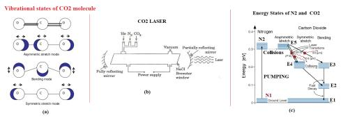
**Figure 7:** Vibrational modes of  $CO_2$  molecule
