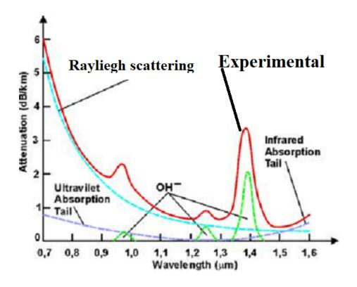
Figure 16: Attenuation in optical fiber
