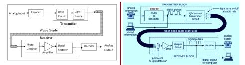
Figure 18: Blocks of Fiber optic communication system
