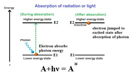
Figure 1: Stimulated absorption of radiation
